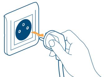
When the plug is removed, the front cover automatically returns to position.
