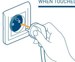
The front cover only moves back when a plug is inserted.
